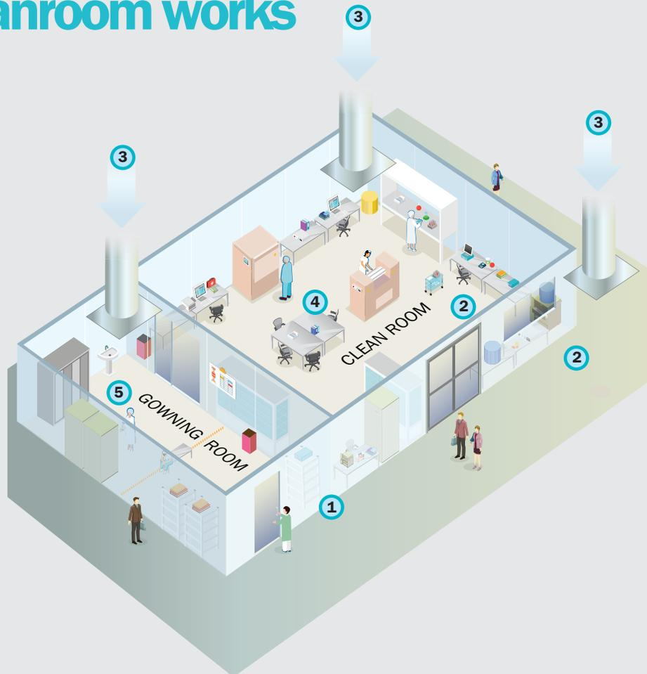
**1** A cleanroom is a controlled environment where products are manufactured. It is a room within a room in which the concentration of airborne particles is controlled to specific limits.
